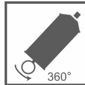
3. Rotate the ring 360° to open the inner cartridge, releasing the hardener
