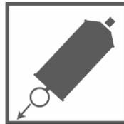
2. Take out the metal ring and insert through the metal pin, pull the ring until it can't go any further
