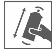
4. Shake the can vigorously for 3 min to mix the components
