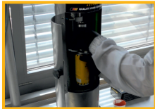
Insert can and cylinder into unit using both hands.
