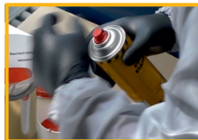
Fit nozzle immediately with slight twisting movement.
